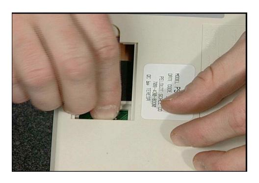
Gently press down to seat the chip into the socket.
